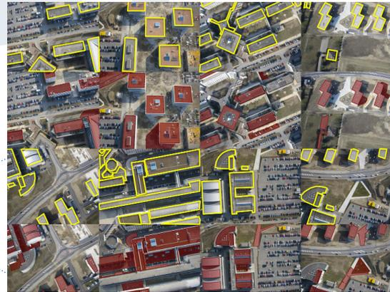
Automatic rooftop detection with our landing place assessment algorithm. Ground-truth annotations are shown in yellow and rooftops detected with our algorithms in red. (image: EPFL)
