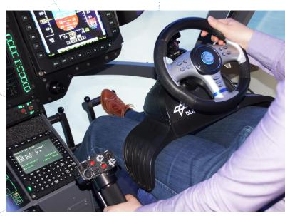
A car-like steering concept in the Flying Helicopter Simulator (Images: DLR)
