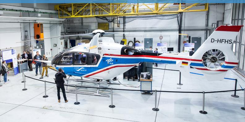
DLR's Flying Helicopter Simulator (ACT/FHS) is a modified EC135 helicopter that can simulate other aircraft in real flight. Within myCopter it was used to investigate the flight dynamics and human-machine interface of a future PAV. The cockpit was equipped with a highway-in-the-sky display and a steering wheel for intuitive car-like control. This is the first helicopter to be flown with a steering wheel. Watch a video [here](#).
