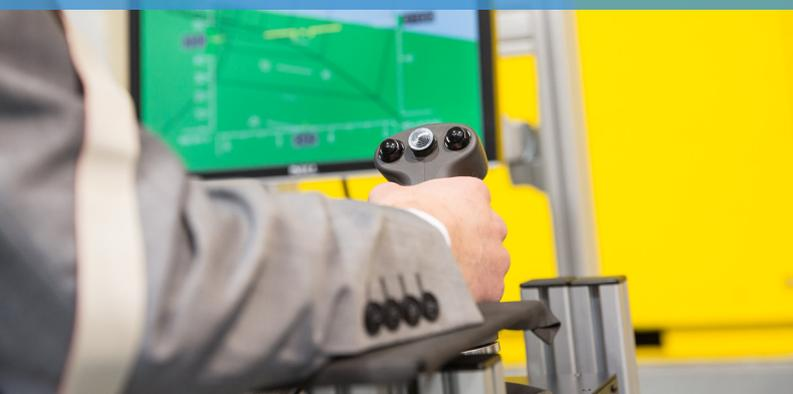
We combined a highway-in-the-sky displays with a haptic shared control framework to assist a non-expert pilot with force guidance cues during a flight through a tunnel trajectory. We have shown that this combination provides an easy-to-use control interface for flying a PAV. Participants could experience this for themselves in a fixed-base simulator. Watch a video [here](#).
