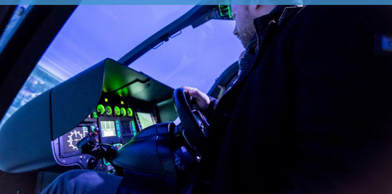
The helicopter simulator of the AVES simulator center was used for ground-based simulation and preparation of FHS flight tests. As in the real helicopter the cockpit was equipped with steering wheel and highway-in-the-sky display. The flight dynamics of a future PAV were simulated and guests could take a flight. Watch a video [here](#).
