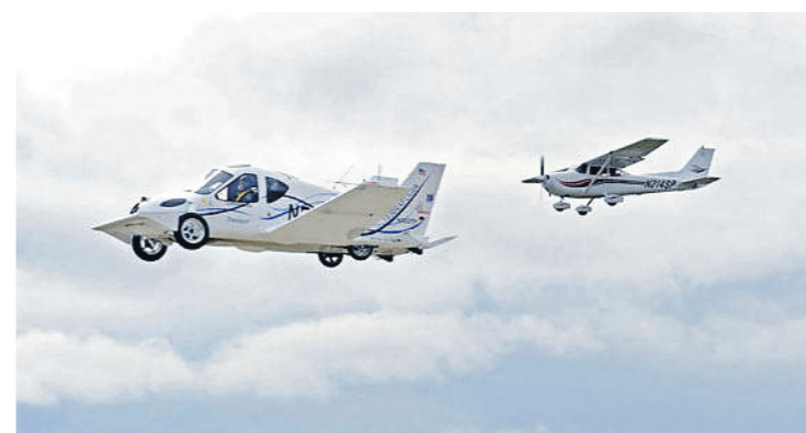
Transformer: With foldable wings the Terrafugia Transition can be used on roads as well as in the air.
