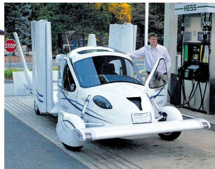
Transformer: With foldable wings the Terrafugia Transition can be used on roads as well as in the air.
