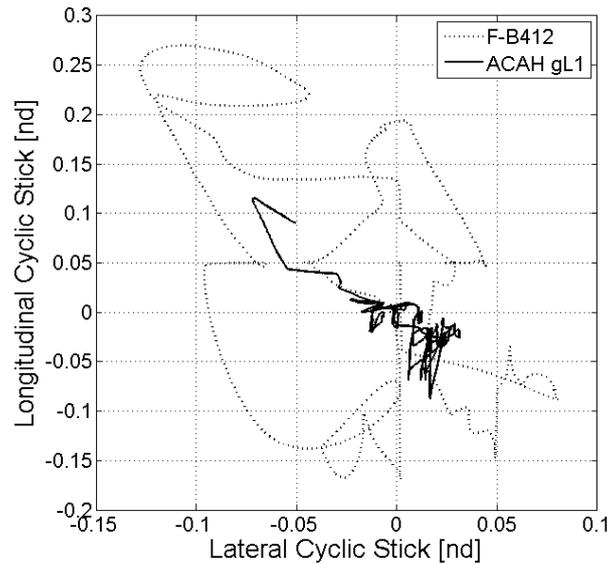
**Figure 7.1: Lateral and longitudinal cyclic activity during a hover task**
