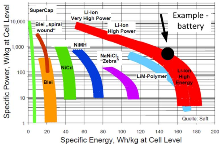
**Figure 5.1: Energy densities of existing batteries with example battery selected for PAV usage [10]**
