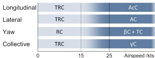
**Figure 8.5: Hybrid response type configuration for PAV usage**
