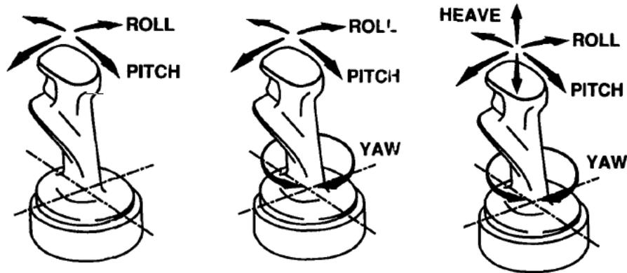
Figure 9.1a, b, c: 2DoF, 3DoF, and 4DoF controller [23]
