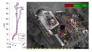
Fig. 2. Altitude test: At  $z \approx 8$  m we switch to vision-based navigation (using sensor feeds from a monocular camera and an IMU only) and fly up to 70 m without intended lateral motion. Then, we let the helicopter descend while applying lateral motion to show the maneuverability during this drastic height change. At the end of the trajectory in the graph, successful vision-based landing is shown, still using only the sensor feeds from the camera and the IMU.
