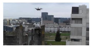
Fig. 1. The MAV operating in a desaster area, only using measurements from a monocular camera and IMU for localization
