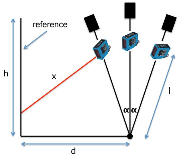
Figure 2: Schematic representation of the relation between the linear distance measurement( $x$ ) and the angular displacement ( $\alpha$ ).
