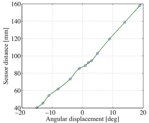
Figure 5: Relationship between the longitudinal angular displacement of the cyclic and the measured linear distance.
