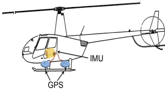
Figure 1: IMU and the GPS antennas position in the lateral view of the R44 helicopter. Modified picture from the "R44 II Pilot's Operating Handbook, Robinson Helicopter Company, 1992".
