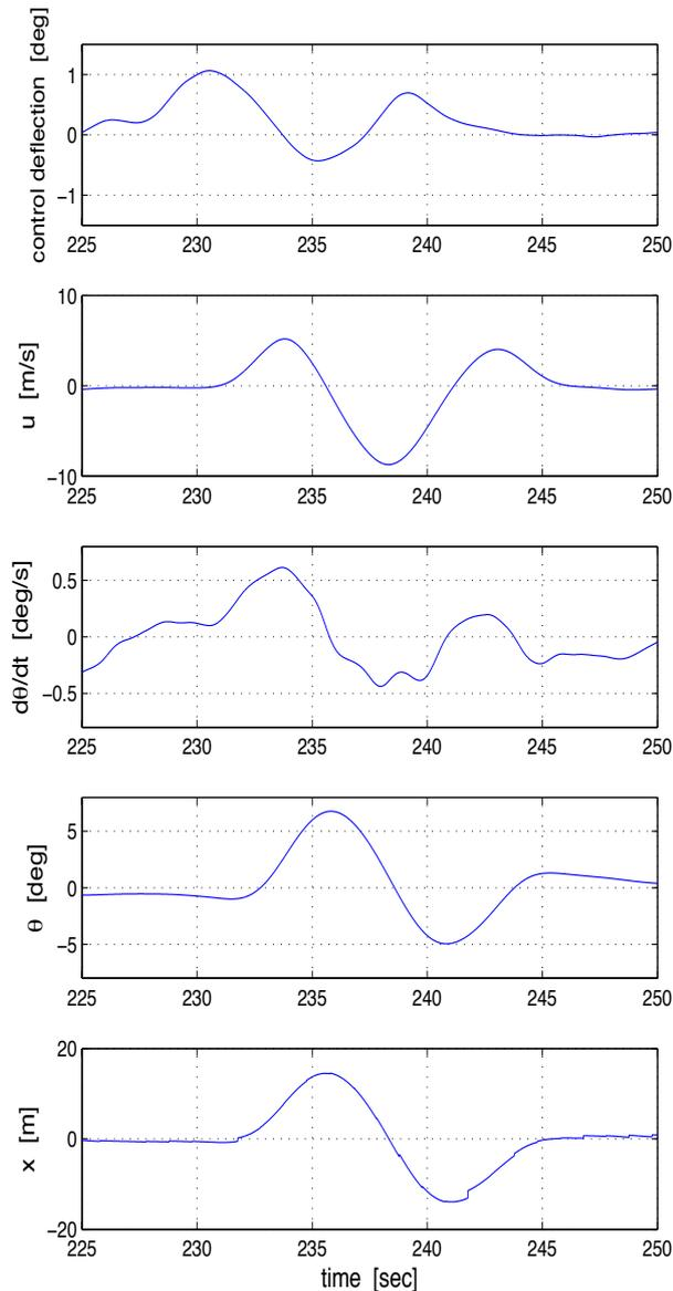
Figure 7: Doublet for the longitudinal axis of the cyclic stick.
