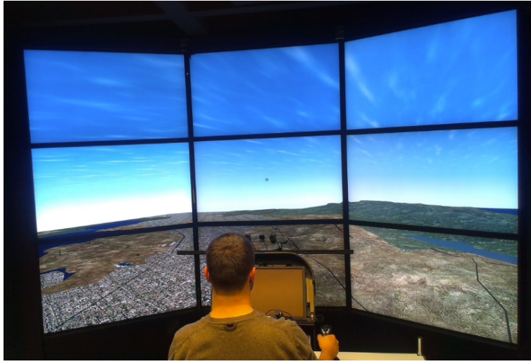
Figure 3. Fixed-base flight simulator, consisting of nine panels and a field-of-view of 105^\circ \times 100^\circ . Here the Outside View is shown. During the experiment, visual disturbances were experienced in the roll-axis around the horizon, that our participants were instructed to compensate for with the provided joystick
